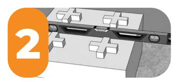
Place your first block. leave a gap of 5mm between the front of the block and the string line. Ensure the block is level in both horizontal directions.
