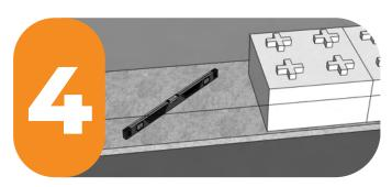
If required, use the long level to smooth out more of the levelling fines. Check it is level in both horizontal directions.
