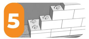
Once you have placed 3 to 4 base blocks, return to the start of the wall to place the remaining layers. Simply stack the blocks on top of each other in a running bond pattern.
