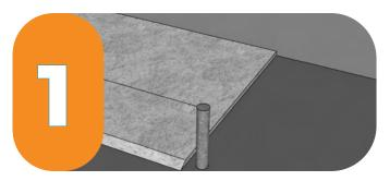
Level the hanging string along the wall. Check level for fines in placement area.
