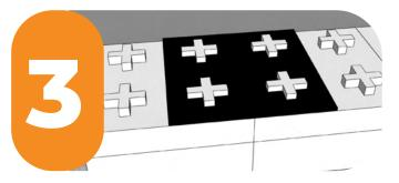
Placed the next block using the stencil to ensure the correct spacing has been achieved. Achieving the correct spacing is the most critical part of the installation process
