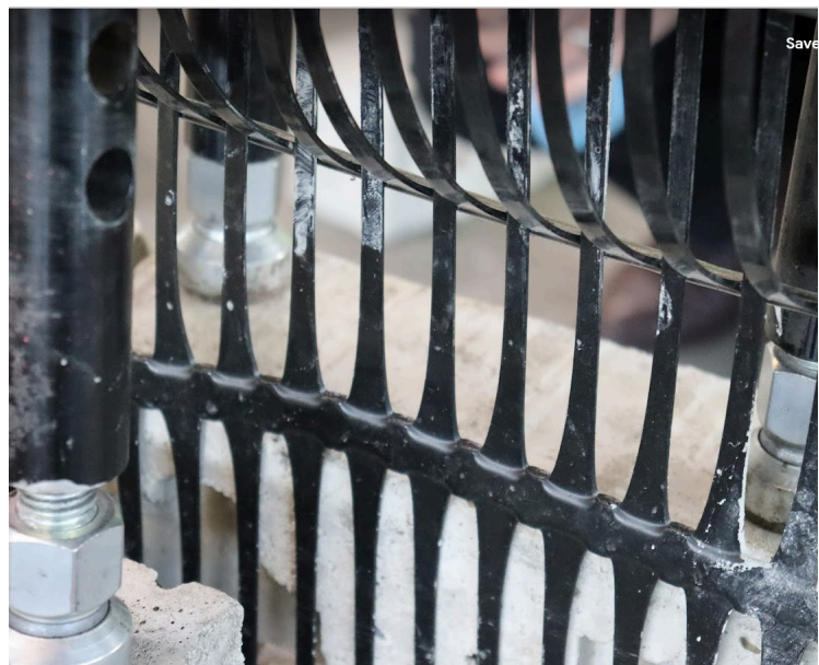
The middle part of the geogrid at 80 kN
